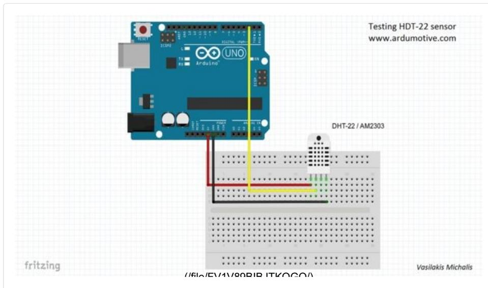
The connections are pretty easy, see the image above with the breadboard circuit schematic.
