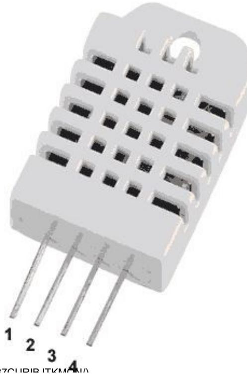
The DHT22 is a basic, low-cost digital temperature and humidity sensor. It uses a capacitive humidity sensor and a thermistor to measure the surrounding air, and spits out a digital signal on the data pin (no analog input pins needed).
